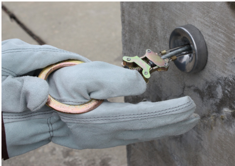
Apply linear pressure to the align trigger block
