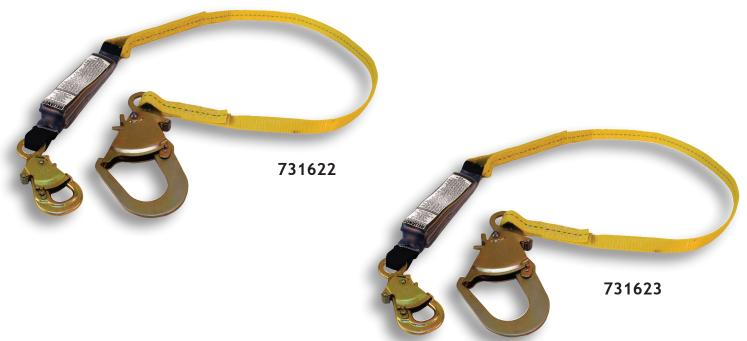
The QuickStop™ series of shock absorbing lanyards is "Tuned" to greatly reduce deceleration distance in the event of a fall. These lanyards are designed for use in areas where clearance to the next lower level is less then 14' (4.2m). Maximum Arresting Force (MAF) will not exceed 1800 lbs (8kN). Steelhead® hooks are for attaching to the back D-ring, and Steel Rebar snap assembly is for anchorage connection.
