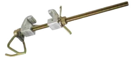
Adjustable Bypass Anchor 3091-1 Temporary HLL Bypass Clamp. Fits I-Beams with 4" -16-5/8" flanges & 1/2" - 1-3/4" flange thickness.
