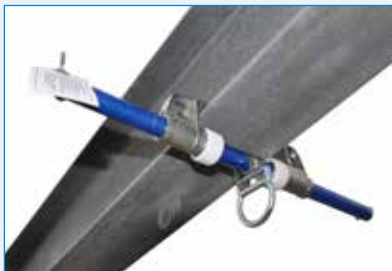
Adjustable Sliding Beam Anchor 3096-1 Fits flange 3-3/4" - 12-1/2" wide & 1/4" - 1-1/4" thick
