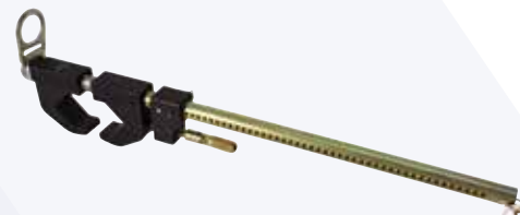
Screwjack™ Adjustable Beam Anchor 3102-1 Fits flange 5-1/4" - 24" wide & 1/4" - 3" thick
