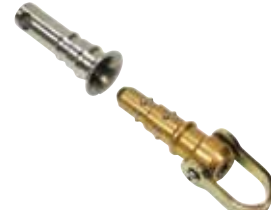
Concrete Embed Anchor 2260-1 Available in carbon or stainless steel. Provides up to 10,000 lb. anchor when attached to receiver. May be used for one or two man anchor or to anchor horizontal lifelines.
