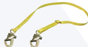
Adjustable Lanyard 717106 3.5' - 6', 1" polyester, 2 ea 3/4" snap hooks
