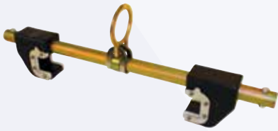
Adjustable Sliding Beam Anchor 3096-1 Fits flange 3-3/4" - 12-1/2" wide & 1/4" - 1-1/4" thick
