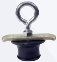
Metal Decking Insert 2243-1 Attaches receiver to 2" holes in decking. Eyebolt used to remove insert after pouring. 2241: Urethane insert only.
