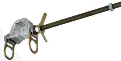
Adjustable Beam Anchor 3098-1 Fits I-Beams with 4" -16-5/8" flanges & 1/4" - 1-3/4" flange thickness, dual anchor rings
